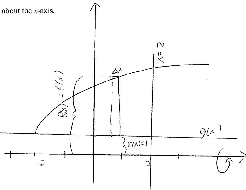
$$\begin{aligned}\Delta V &= \pi [R(x)^2 - r(x)^2] \Delta x \\ &= \pi [(\sqrt{x+2} + 1)^2 - 1^2] \Delta x \\ &= \pi [x+2 + 2\sqrt{x+2} + 1 - 1] \Delta x\end{aligned}$$
