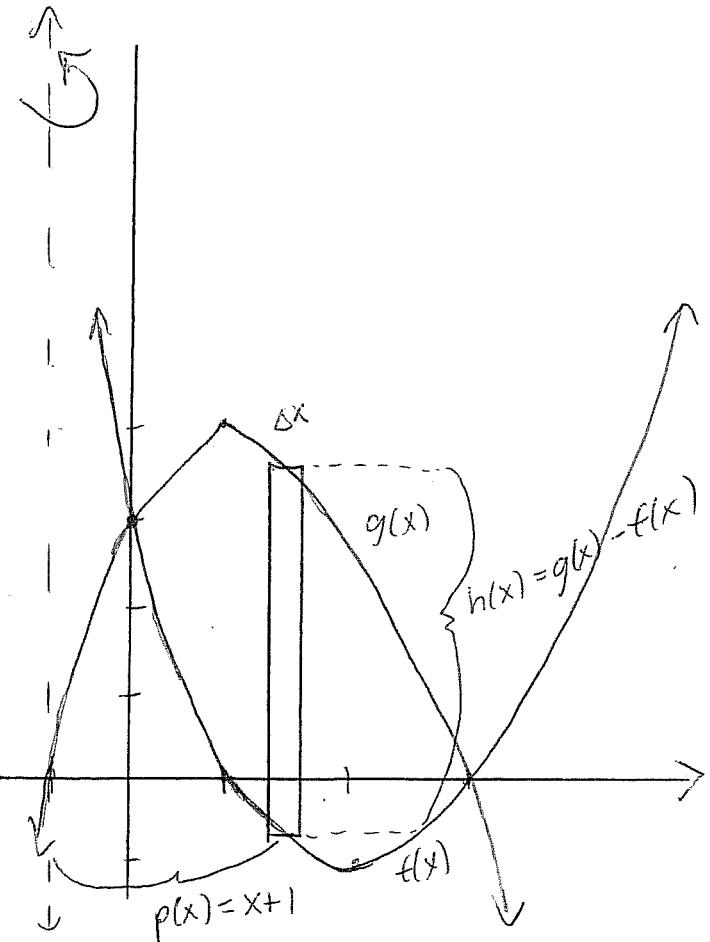
$$\begin{aligned} \Delta V &= 2\pi p(x) h(x) \Delta x \\ &= 2\pi(x+1)(g(x) - f(x)) \Delta x \\ &= 2\pi(x+1)(-x^2 + 2x + 3 - x^2 + 4x - 3) \Delta x \\ &= 2\pi(x+1)(-2x^2 + 6x) \Delta x \end{aligned}$$
