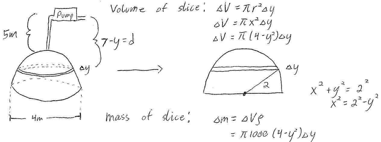
$$\begin{aligned} \text{Force of slice: } \Delta F &= \Delta m g \\ &= \pi 1000 (4 - y^2) (9.8) \Delta y \\ &= \pi 9800 (4 - y^2) \Delta y \end{aligned}$$
