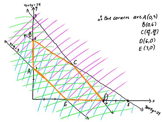
To find C, lets determine the intersection between 3x+4y = 24 and 4x+3y = 24
