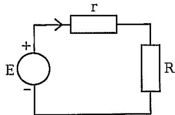
In such a circuit, the electric current  $i$  is given by  $\frac{E}{r+R}$  and the power  $P$  delivered to the load  $R$  is given by  $P = Ri^2$ .
